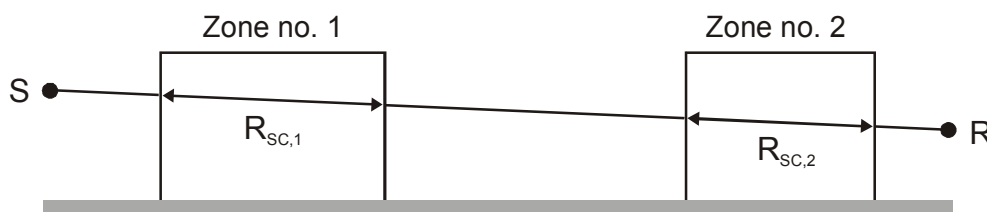
Figure 46 Propagation path used to determine the scattering zone path length R_{sc} when the line-of-sight is unblocked.
