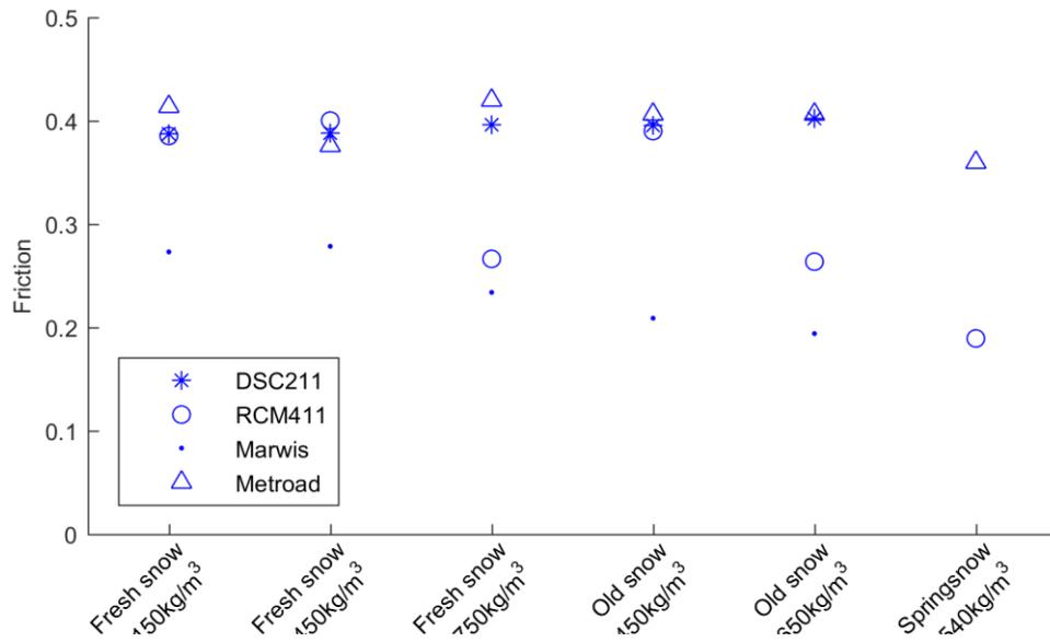
Figure 3 The derived friction values on the different types of snow.
