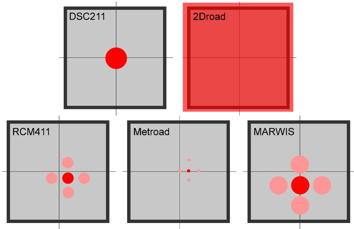
Figure 1 Sensing spots for the different sensors. For the mobile sensors, the red circle indicates the central spot, while the pink circles show the other four positions where measurements were made.
