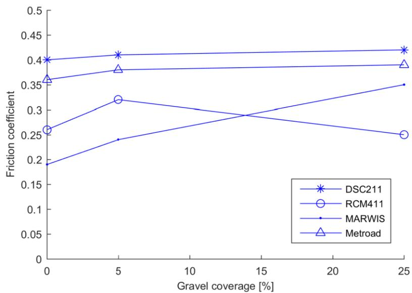
Figure 4 The change of derived friction coefficient as a function of the amount of gravel coverage on compacted snow.
