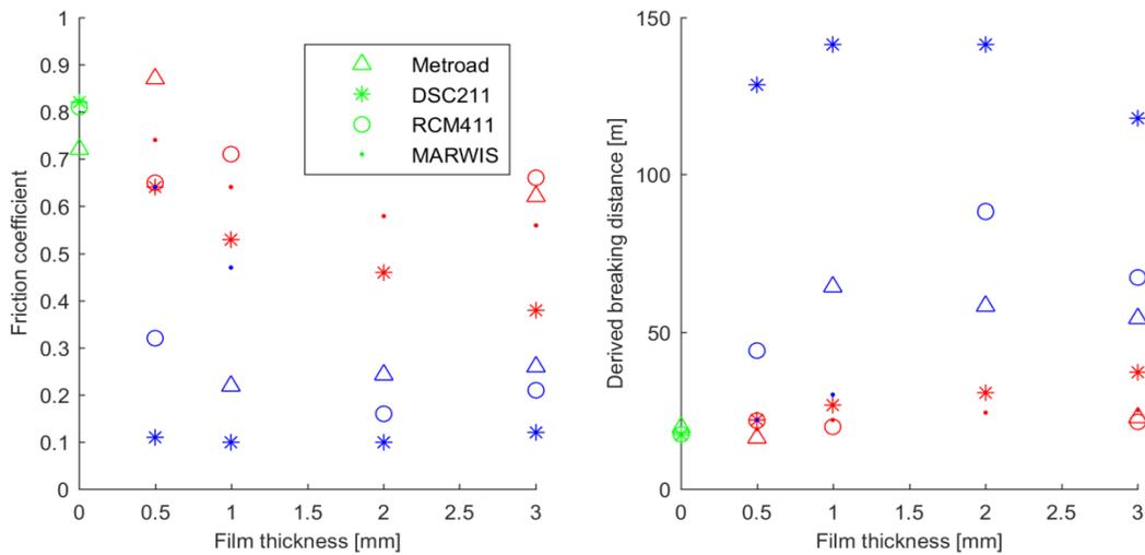
Figure 2 a) Friction coefficient provided by the different sensors on films of water (red markers) and ice (blue markers). The dry asphalt reference is given as a 0 mm film thickness (green markers). b) Shows the derived breaking distance from the acquired friction coefficients, assuming a velocity of 60 km/h.
