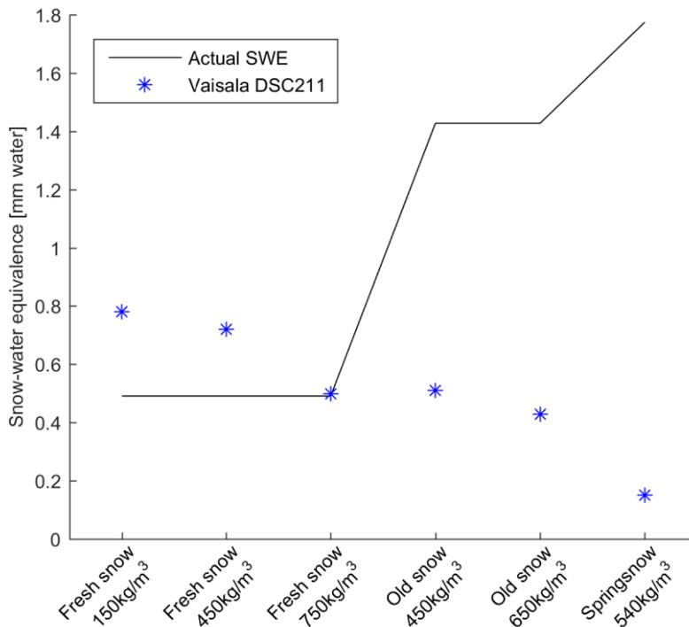
Figure 7 Measured snow-water-equivalence for the different snowtypes and densities
