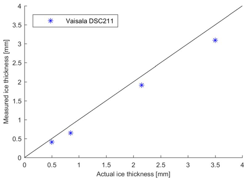
Figure 6 Ice film thickness measured by the DSC211. The black line indicates a 0% measurement error.
