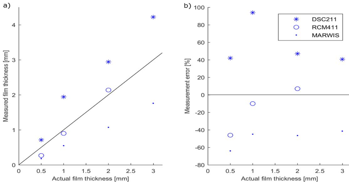
Figure 5. The water film thickness on the gray asphalt measured by three of the sensor, a) as a function of actual water film thickness and b) the corresponding error of the measurements.
